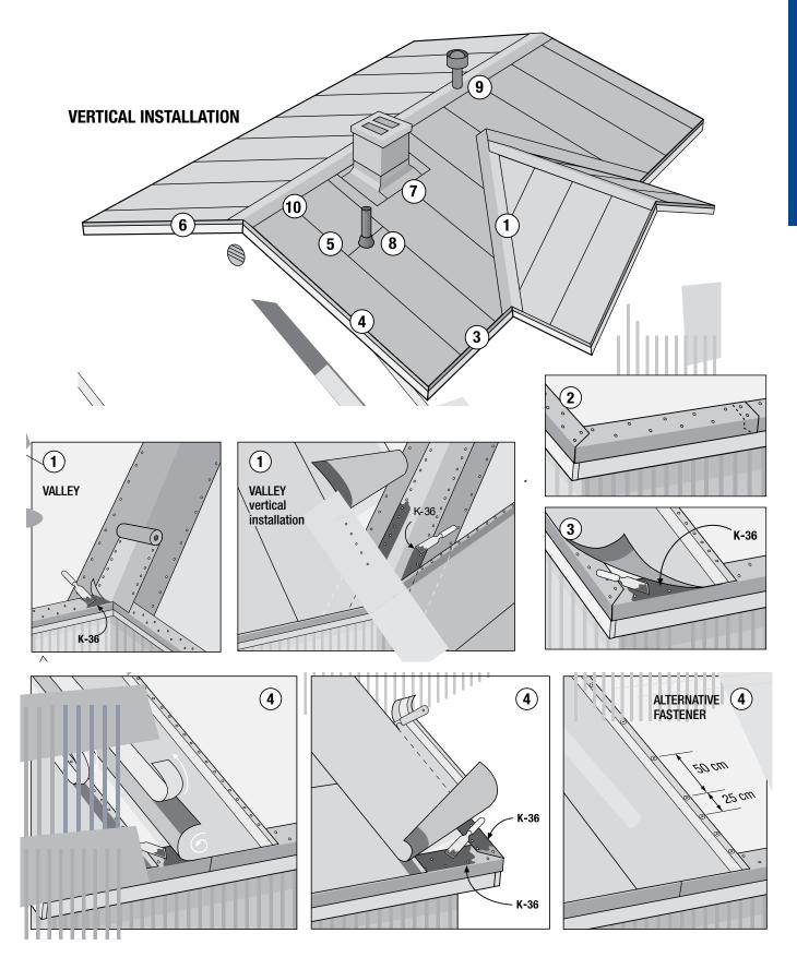
Self-adhesive cap sheet with SBS elastomer bitumen  $1 \times 7 \text{ m}$
